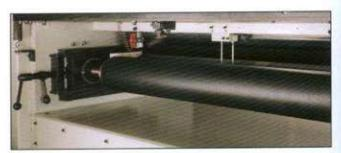
SHOWN ABOVE: Easy accessibility to the glue print cylinder makes set-ups and clean-ups simple and fast.
