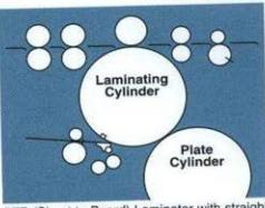
STB (Sheet to Board) Laminator with straight paper line for heavy board stock with registration +/- .040" (1mm)
