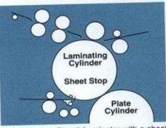
STS (Sheet to Sheet) Laminator with a sheet stop on the laminating cylinder for precision registration +/- .015" (0.375mm)
