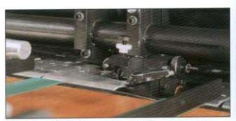
SHOWN ABOVE: A cam driven pinch roll pulls each sheet to its final side registration. Individual cam driven pinch and acceleration rolls then advance the sheet to the laminating cylinder.
