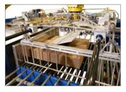
Optional automated tie sheet placement between desired layers.
