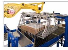
A picked layer with tie sheet being positioned to form a load.
