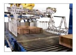
The MasterStak Palletizing Robot straightens and stacks layers to form the most stable load configuration.
