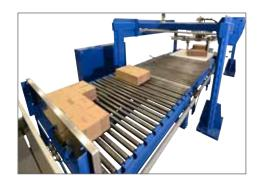
The MasterStak Positioning Robot translates and rotates bundles into an unlimited number of layer configurations. Servo controlled positioning provides push-button size and layering change overs.
