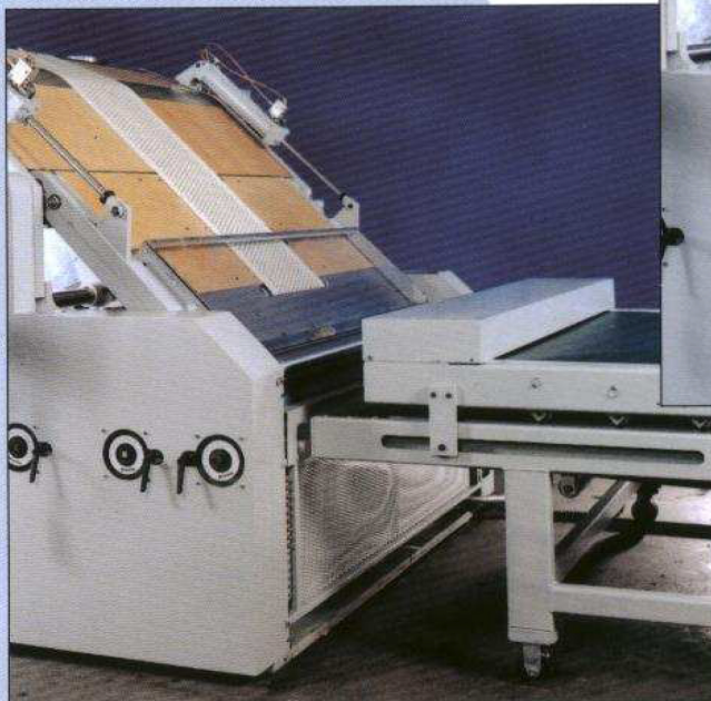
ABOVE: Operator accessibility is a key feature of the NEWPAKS®. The feed table flips up and out of the way by pushbutton, and the compression section is easily rolled back for convenient access to the laminating section.
