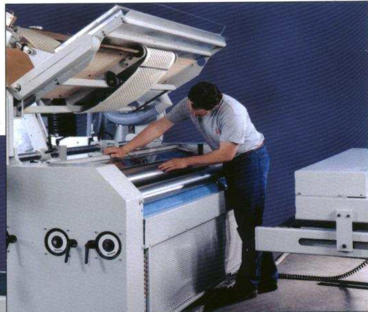
ABOVE: Operator accessibility is a key feature of the NEWPAKS®. The feed table flips up and out of the way by pushbutton, and the compression section is easily rolled back for convenient access to the laminating section.
